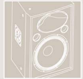
Trapezoidal designs allow more compact arrays and sonic accuracy
